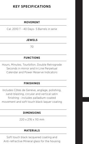
Anti-refractive Mineral glass for the housing 50.6593/201: Palladium coated movement 50.6593/221: Palladium coated Wheel and Black Gold Main plates coating for the movement
